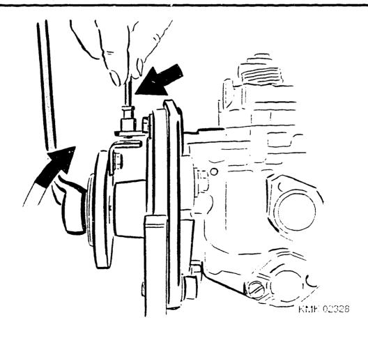
Tighten fastening screws of upper notched plate.
